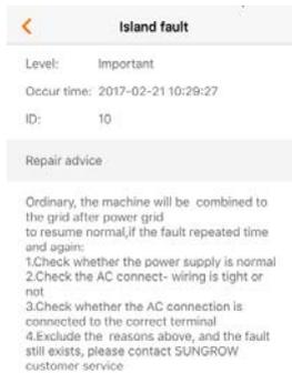
**Fig. 10-11** Detailed fault alarm info
