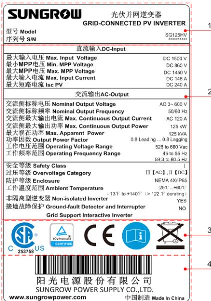
Fig. 4-2 Inverter nameplate
