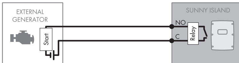
Figure 11: Connecting the Generator Control to Sunny Island
