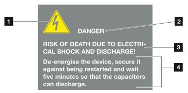
Fig. 4: Structure of the warnings
