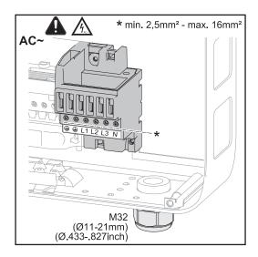
PE Ground conductor / grounding
