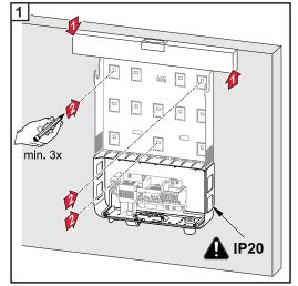
Tip: Install the inverter such that its display is at eye level
