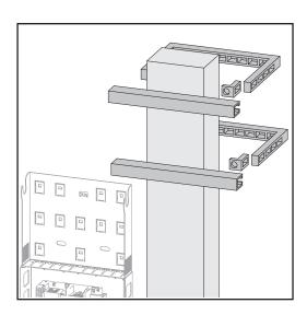
When installing the inverter on a mast or support, Fronius recommends the "Pole Clamp" kit from Rittal GmbH (order no. SZ 2584.000).
