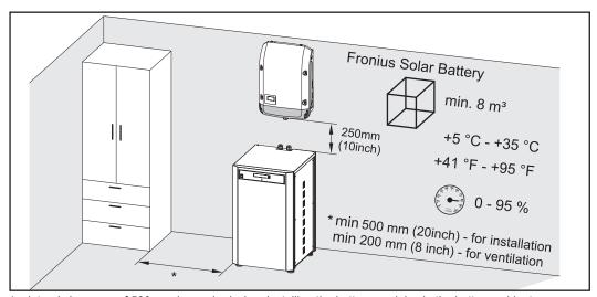
$^{\star}$  a lateral clearance of 500 mm is required when installing the battery modules in the battery cabinet
