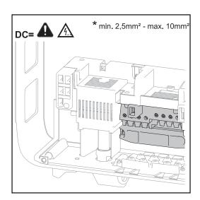
Max. cross-section of each DC cable: 10 mm<sup>2</sup>
