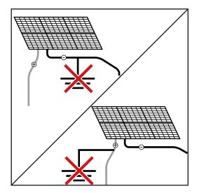
The Hybrid inverter is a transformerless device. The individual poles of the solar modules must not be grounded.
