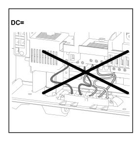
If DC cables are laid over the shaft of the DC main switch or across the connection block of the DC main switch, they may be damaged when the inverter is swung in or they may even prevent the inverter from being swung in.
