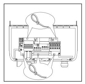
If overlength AC or DC cables are to be laid in loops in the connection area, attach the cables with cable ties to the eyelets provided on the top and bottom of the connection block.
