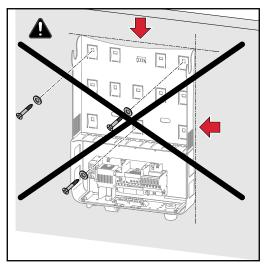
Fixing the mounting bracket to a wall
