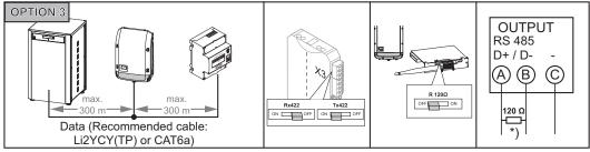
\* The terminating resistor is included with the Fronius Smart Meter
