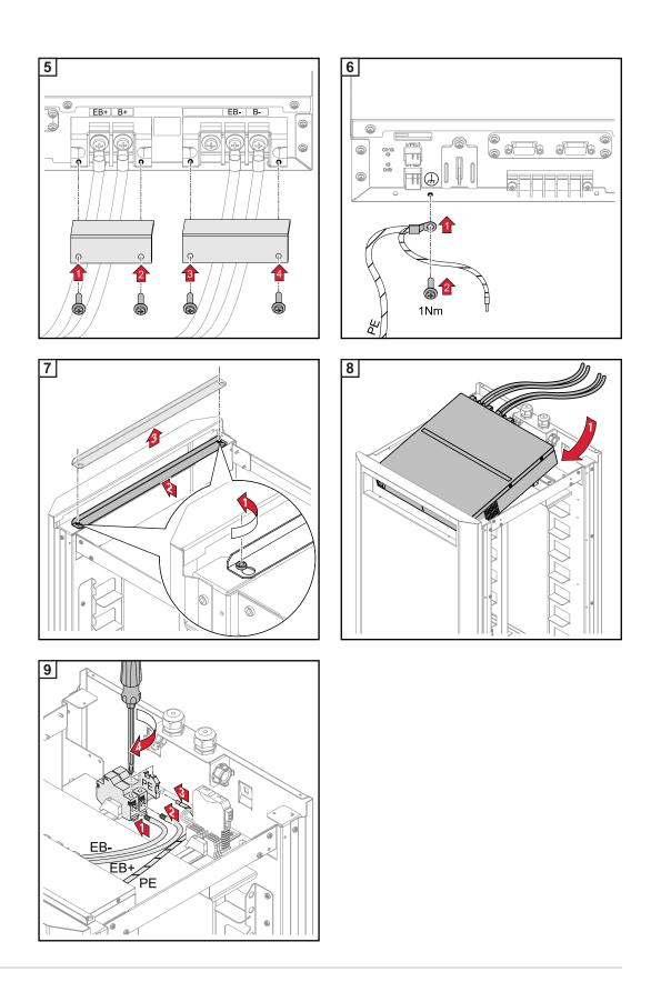
Installing the battery modules in the battery cabinet
