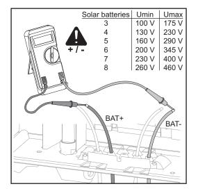
IMPORTANT! Check the voltage of the battery modules.
