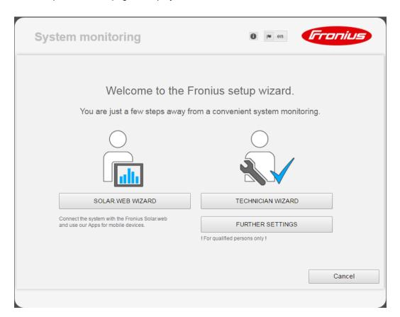
If you run the technician wizard, always remember to make a note of the assigned service password. This service password is required to enter settings in the "System overview" and "DNO Editor" menus as well as for advanced battery settings.
