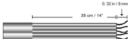
Figure 33: Insulation stripping – AC
