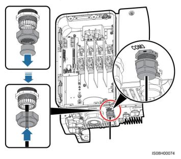
**Step 3** Loosen the minus screw on the cable connector, and connect the solar tracker power cable.
