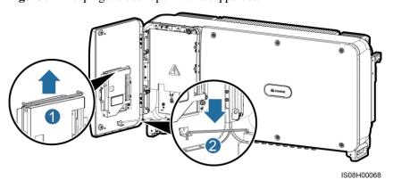
**Step 3** Remove the cover and hang it on the hook of the door.
