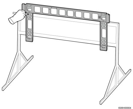
Figure 4-10 Determining hole positions
