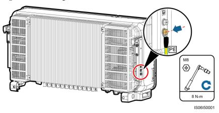
**Step 3** (Optional) To enhance the corrosion resistance of a ground terminal, apply silica gel or paint around the terminal.
