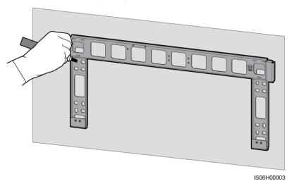
Step 2 Drill holes using a hammer drill and install expansion bolts.
