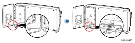
**Step 3** Close the maintenance compartment door and tighten the two screws on the door.
