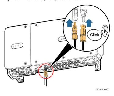
Figure 5-21 Connecting DC input power cables
