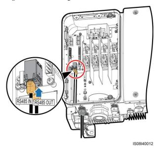
Figure 5-33 Connecting communications cables
