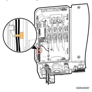
**Step 6** Tighten the thread-lock sealing nut and seal the cable gland.
