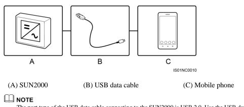
The port type of the USB data cable connecting to the SUN2000 is USB 2.0. Use the USB data cable delivered with the mobile phone.
