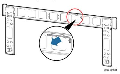
Figure 4-9 Removing a security torx wrench
