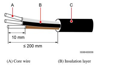
**Step 2** Route the cable through the cable gland.
