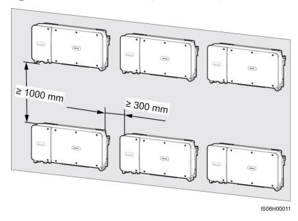
Figure 4-7 Stacked installation mode (not recommended)
