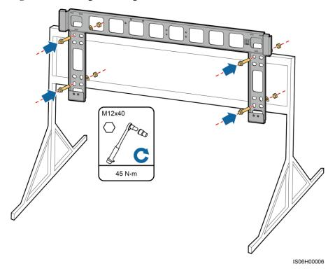
Figure 4-12 Securing a mounting bracket
