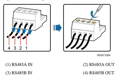
Step 4 Land the cables in the terminal block, and bond the shield layer to the ground point.
