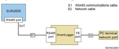
Figure 5-22 Communication mode for a single SUN2000
