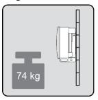
• In residential areas, do not install the SUN2000 on drywalls or walls made of similar materials which have a weak sound insulation performance because the noise generated by the SUN2000 is noticeable.
