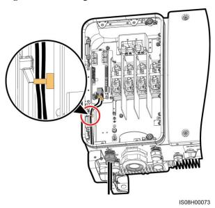
**Step 5** Tighten the thread-lock sealing nut and seal the cable gland.
