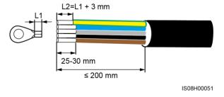
Step 4 (Optional) Crimp an OT terminal on the PE cable.
