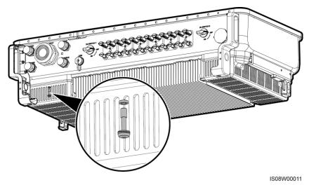
**Step 2** Open the maintenance compartment door and keep it open with the support bar.
