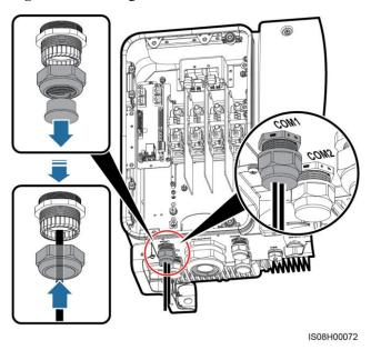
**Step 3** Insert the RJ45 connector into the RJ45 network port in the SUN2000 maintenance compartment.
