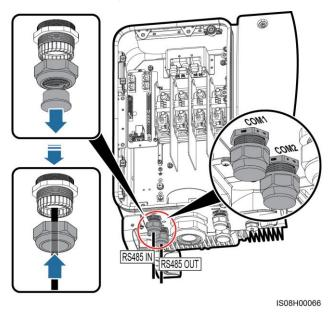
**Step 3** Remove the cable terminal base from the terminal block, and connect the communications cable to the terminal base.
