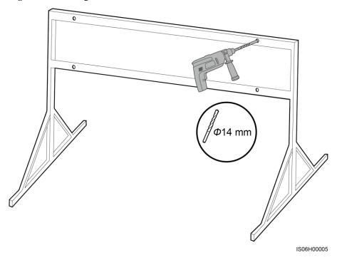
**Step 3** Align the mounting bracket holes with the drilled holes, insert bolt assemblies (flat washers, spring washers, and M12x40 bolts) into the holes through the mounting bracket, and secure them using the supplied stainless steel nuts and flat washers.
